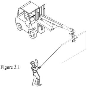
Step 4: Remove the device out of the stone slab.
