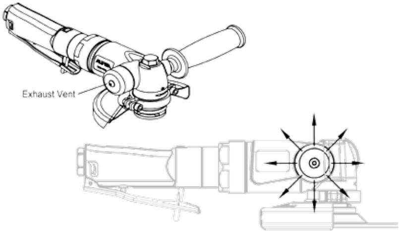
The exhaust vent cover can be rotated 180 degrees to divert the air flow coming out of the Pneumatic Angle Grinder.
